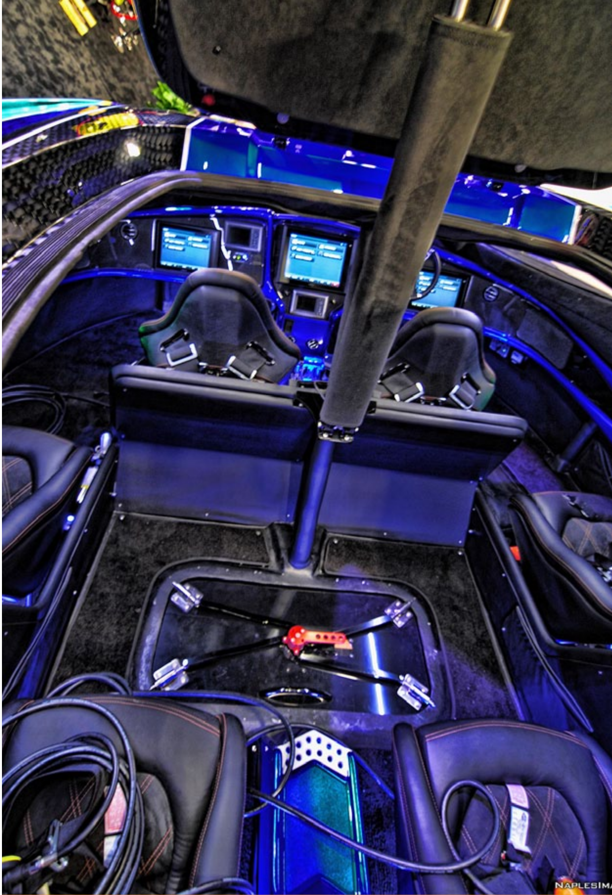
Each of the cat's six bucket seats in the uniquely configured cockpit has a five-point restraint harness as well as its own emergency oxygen system.
