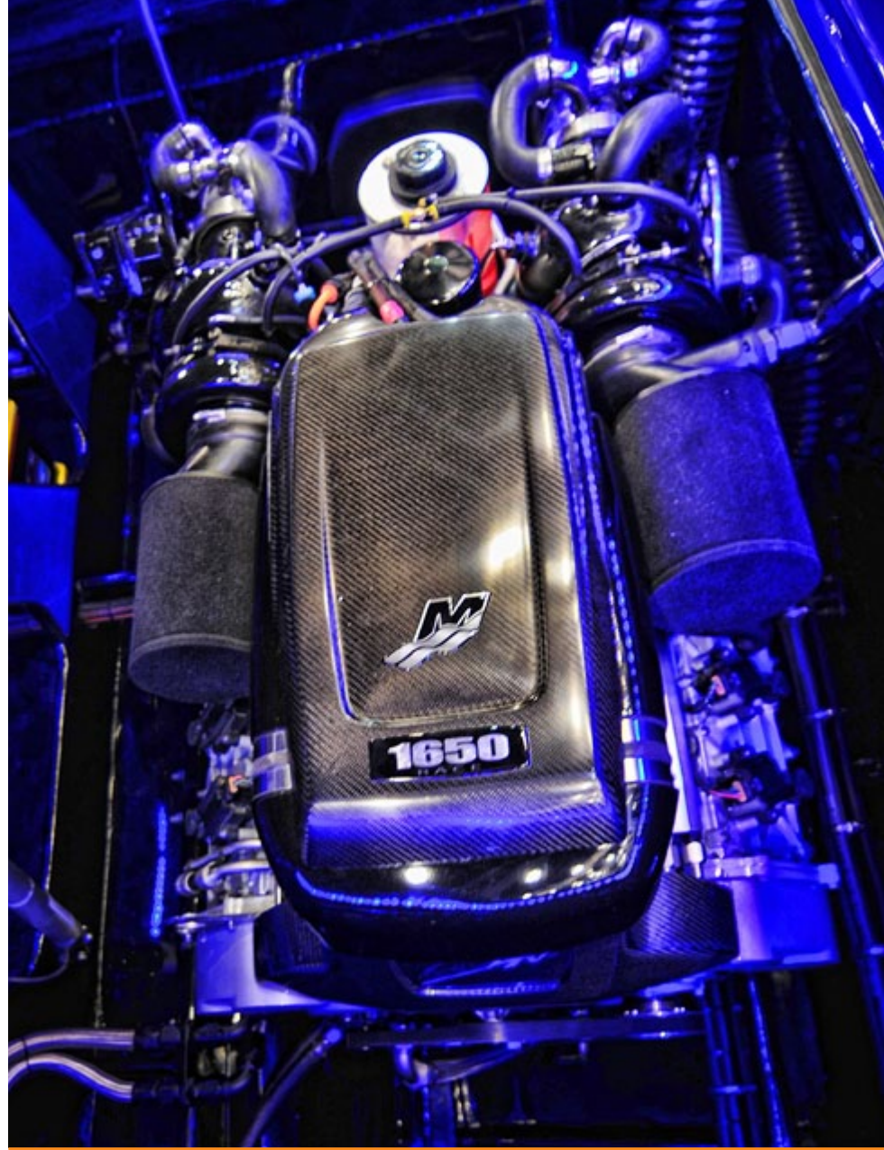
A pair of 1,650-horsepower turbocharged beauties from Mercury Racing powers the show-stopping 52-foot cat.
